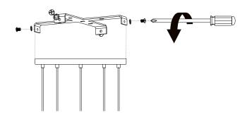
Remove the fixing screws and mounting bracket (B) from ceiling cup and retain for later use.
