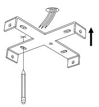
Using the bracket (B) as a template, mark and drill fixing holes in the ceiling. Due to the variety of different ceiling types Soho Home cannot provide you with the exact fittings needed to fix this product to the ceiling. Different materials require different types of fittings.
