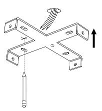
Using the bracket (B) as a template, mark and drill fixing holes in the ceiling. Due to the variety of different ceiling types Soho Home cannot provide you with the exact fittings needed to fix this product to the ceiling. Different materials require different types of fittings.
